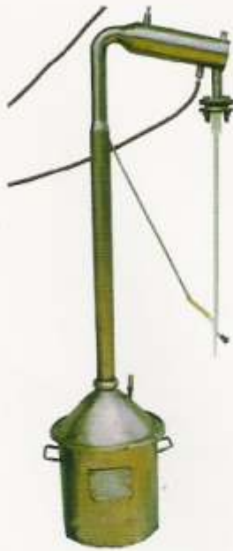
Mini Essential Oil Distillation Apparatus
